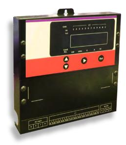
IPP series is a single/three phase remotely monitored power meter, built-in 12 independent measurement modules. User may select any one phase of the input voltage as a measurement reference. It supports the monitoring of twelve loops of 1P2W, or four loops of 3P3W/3P4W, or a hybrid combination, providing flexible application.
