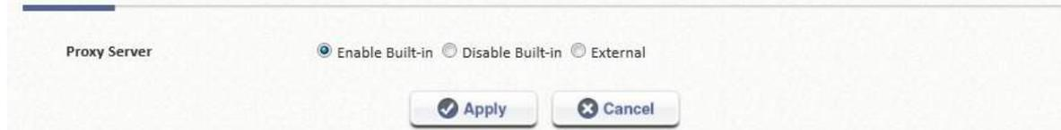
Step 6. Select **Enable Built-in** and click **Apply** to save the settings
