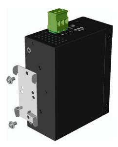
2. Attach bracket to the lower edge of the DIN rail and push the unit upward a little bit until the bracket can clamp on the upper edge of the DIN rail.
