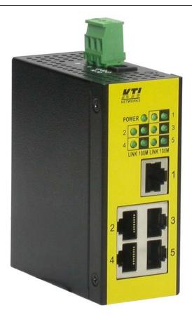
The switch provides five 10/100Mbps copper ports for connections to Ethernet and Fast Ethernet devices. With the featured auto-negotiation function, the switch can detect and configure the connection speed and duplex automatically. The switch also provides auto MDI/MDI-X function, which can detect the connected cable and switch the transmission wire pair and receiving pair automatically. This auto-crossover function can simplify the type of network cables used.
