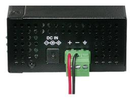
Note: When using terminal block connectors, put a cap on the DC jack.
