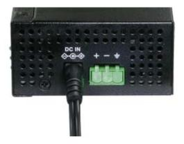
Note: When using terminal block connectors, put a cap on the DC jack.
