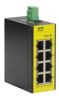
The switch provides eight 10/100Mbps copper ports for connections to Ethernet and Fast Ethernet devices. With the featured auto-negotiation function, the switch can detect and configure the connection speed and duplex automatically. The switch also provides auto MDI/MDI-X function, which can detect the connected cable and switch the transmission wire pair and receiving pair automatically. This auto-crossover function can simplify the type of network cables used.
