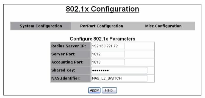
Fig 4.5.2.0 System Configuration
