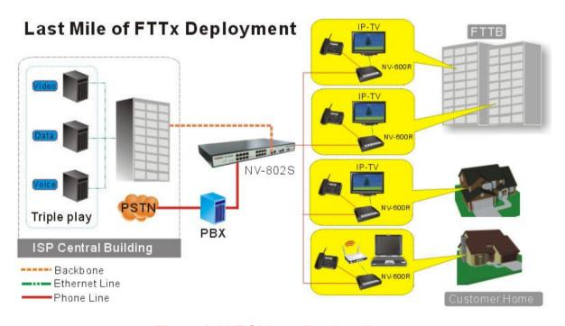
Figure 6.1 VDSL2 application diagram
