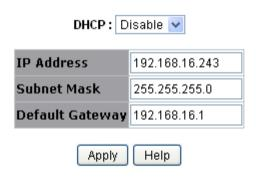
Fig. 4.2.0 IP Address Setting
