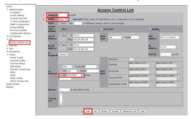
Fig.4.4.0.1 Configure DHCP Block
