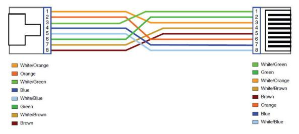
Figure C-3 Pin Assignments and Wiring for an RJ-45 Crossover Cable
