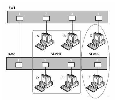
The NV-802S supports both port-based VLAN and tag-based (802.1Q) VLAN modes. The default configuration is tag-based (802.1Q) VLAN. In the 802.1Q VLAN, initially, all ports on the switch belong to default VLAN, VID is 1.
