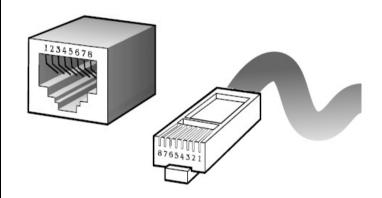
Figure C-1 Standard RJ-45 repectacle/connector
