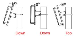
**1.** For +15° and 0° angle installations, position the bracket with the +15° mark on the top.
