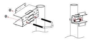
3. Use a wrench to tighten the four nuts onto the screws.
