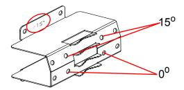
For -15° installation, position the bracket so the -15° mark is on top.
