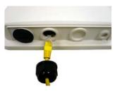
2. Open the claw (B) then close it tightly around the cable.
