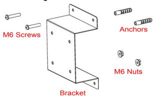
1. Place the bracket where you want it on the wall (W) and mark the position of the outer holes with a pencil. Remove the bracket and drill the holes where marked. Insert the anchors in the holes. Screw the bracket to the wall.
