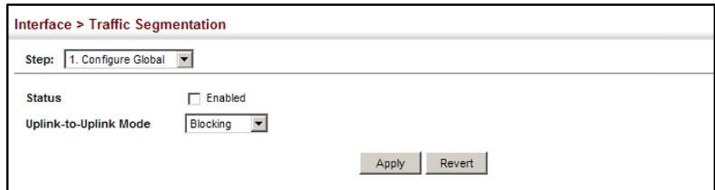
Figure 72: Enabling Traffic Segmentation
