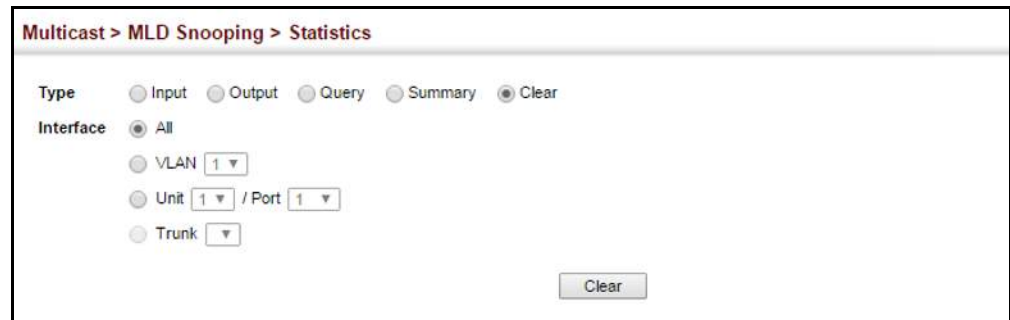
Figure 314: Clearing MLD Snooping Statistics
