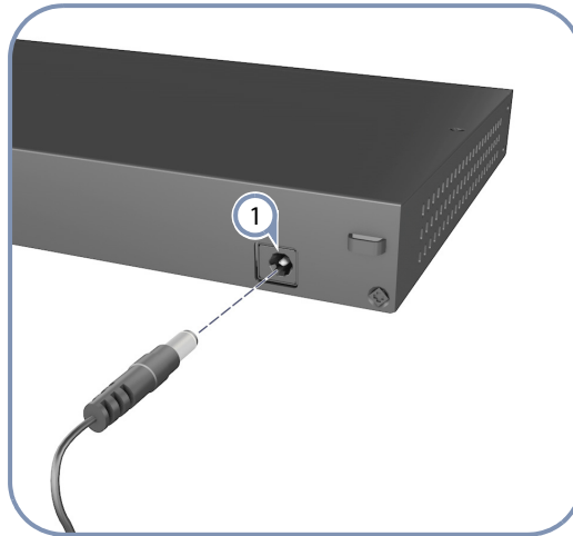
Figure 18: DC Power Cord and Power Socket
