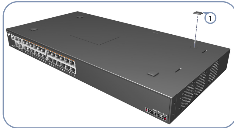
Figure 14: Attaching the Adhesive Feet
