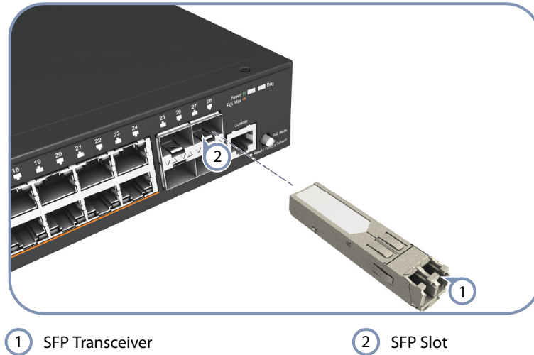
Figure 20: Inserting an SFP/SFP+ Transceiver into a Slot
