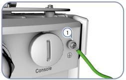
Ground the AP by connecting the included ground wire to the grounding point on the AP and to nearby good earth connection.
