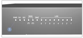
Verify the device is powered on by checking the PWR LED. When operating normally, the PWR LED should be on green.
