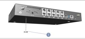
1. Attach the four rubber foot pads to the base of the device, and then place it on a desktop or shelf.
